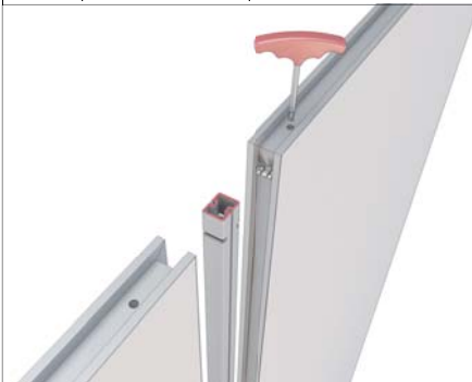
Sketch of panels connection — top structure
