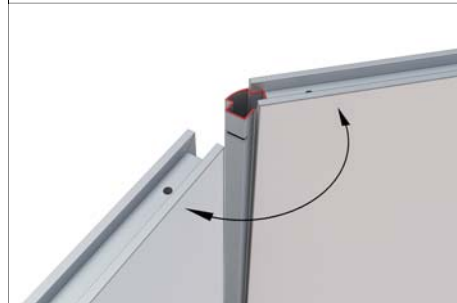
connect with beam by extention extrusion
