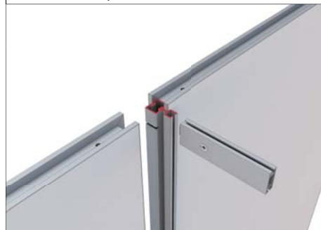
connect with beam by extention extrusion
