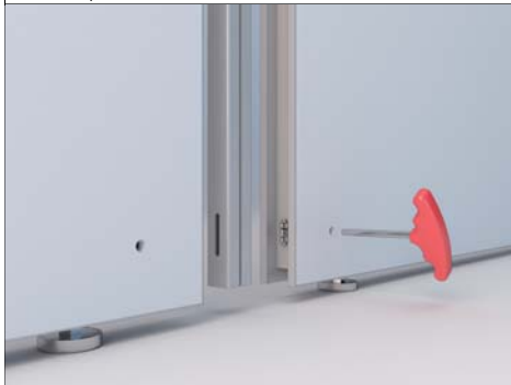
Sketch of panels connection — bottom structure
