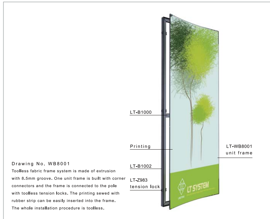
LT-B1002_8.5 double-side fabric extrusion- groove size 8.5mm
